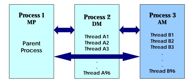
The parent process creates process 2, which in turn spawns threads A1 to A96 in process 2's address space. Thereafter, each of these threads may spawn a corresponding thread B1 to B96 in another process's address space (process 3). Process 3 may possibly be running on a remote CPU.
